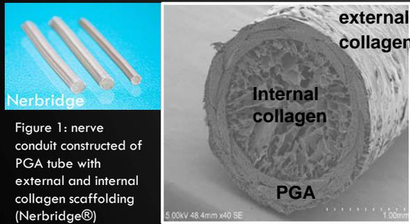
Figure 1: nerve conduit constructed of PGA tube with external and internal collagen scaffolding (Nerbridge®)
