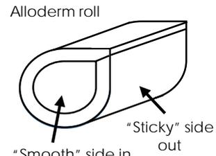
In a large goat model, one AMI was created at the time of primary transtibial amputation. The distal tendon of the *medial gastrocnemius* was passed through a rolled piece of Alloderm, and coapted to the distal *tibialis cranialis*. The Alloderm pulley was then sutured closed, and affixed directly to the surficial fascia via five sutures. Placement of the pulley was selected to preserve biological levels of tension in each muscle.
