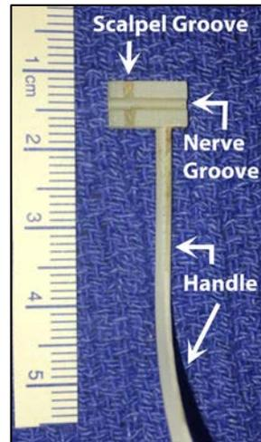
**Figure 1:** Partial cut device with nerve and scalpel grooves. Different devices were used for each of the three different cut depths.
